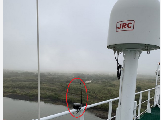
Even though it may seem like a good spot for the CAT MAX, it's actually not ideal because the antennas block a large portion of the sky and may cause interference by emitting high power.
