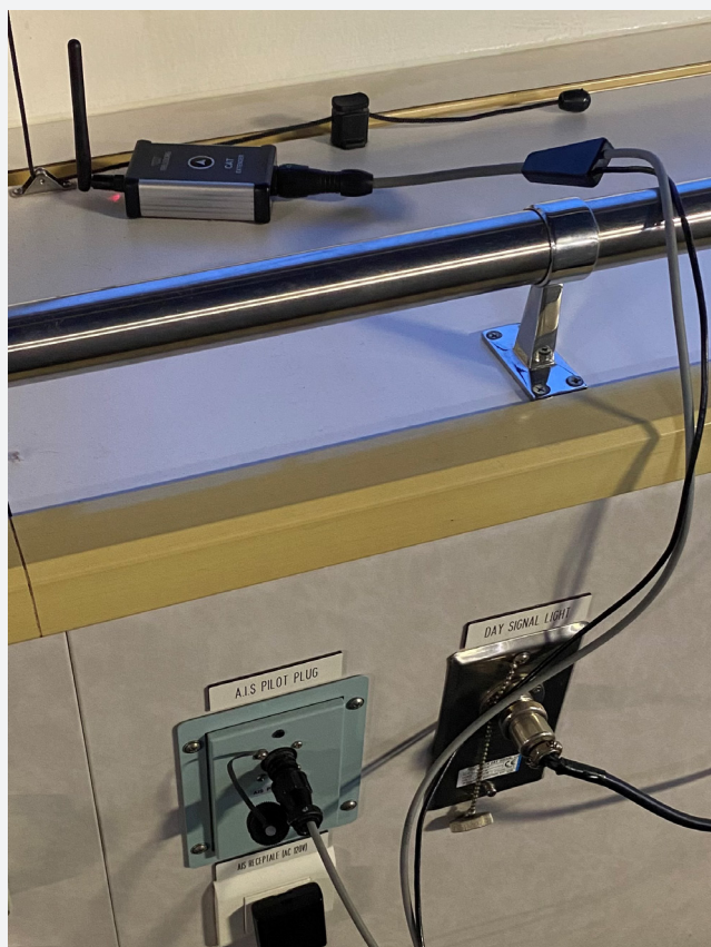
CAT EXTENDER connected to the Pilot Plot
