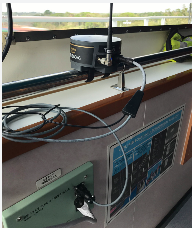
CAT MAX HDG connected to the Pilot Plot
