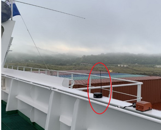
Very good location, as the area around the CAT MAX unit is clear and free of obstacles.
