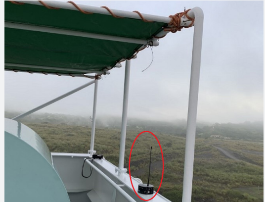
Due to the proximity of numerous metal pipes, this location is not suitable for the CAT MAX.
