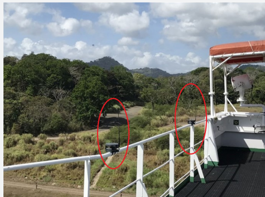
This is a great location for the CAT MAX because the only obstruction to the view of the sky from the two units is the Panama Roof, which is made of plastic and is at a sufficient distance.
