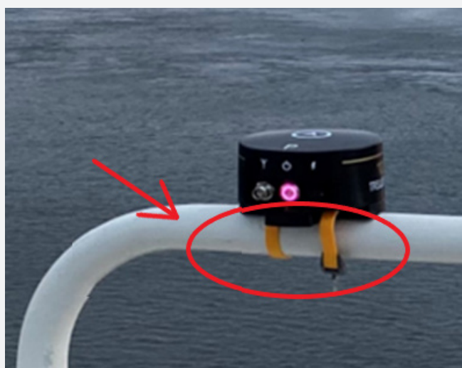
CAT MAX unit mounted on a pipe railing using the included bracket.
