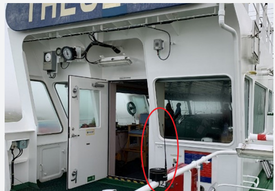
Here, the wheelhouse is too close to the CAT MAX unit, blocking almost half of the sky view, making it less suitable for placement.
