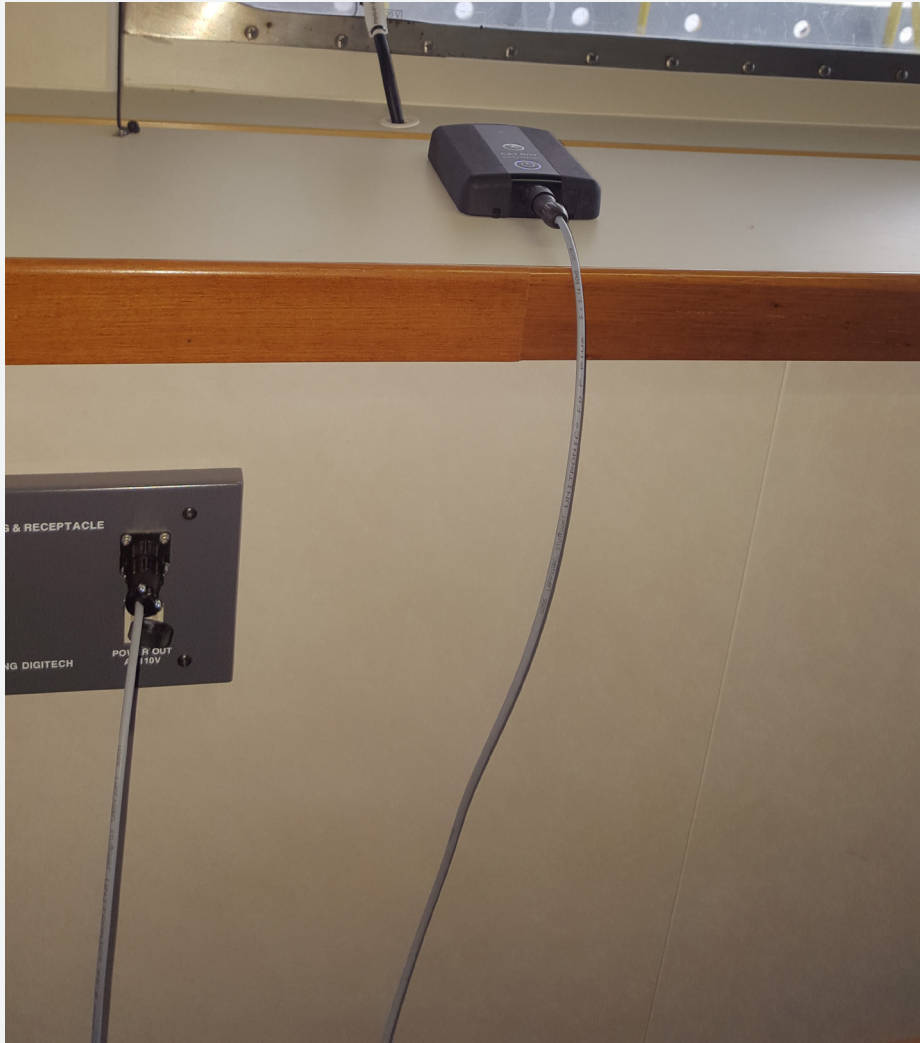
CAT ROT is connected to the pilot plug and placed on a horizontal surface.
