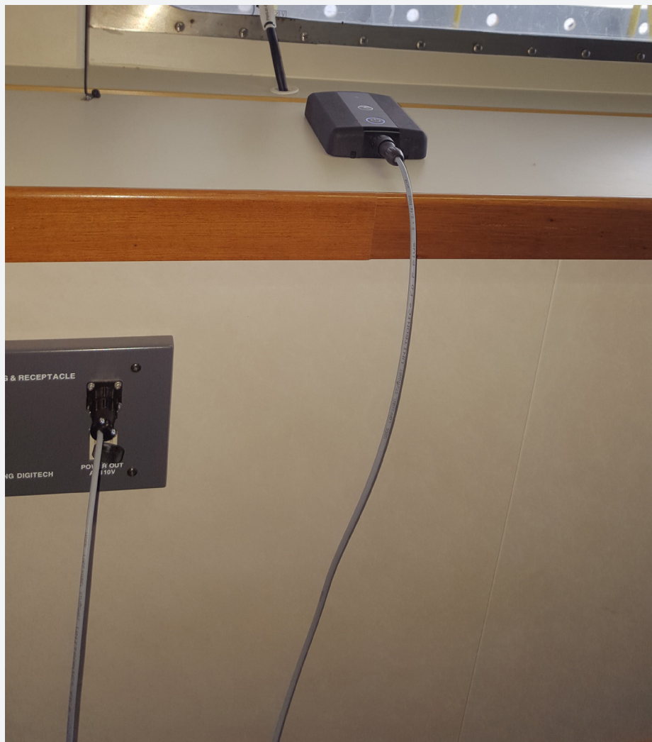
CAT XT AIS, connected to the pilot plug and placed on a horizontal surface.
