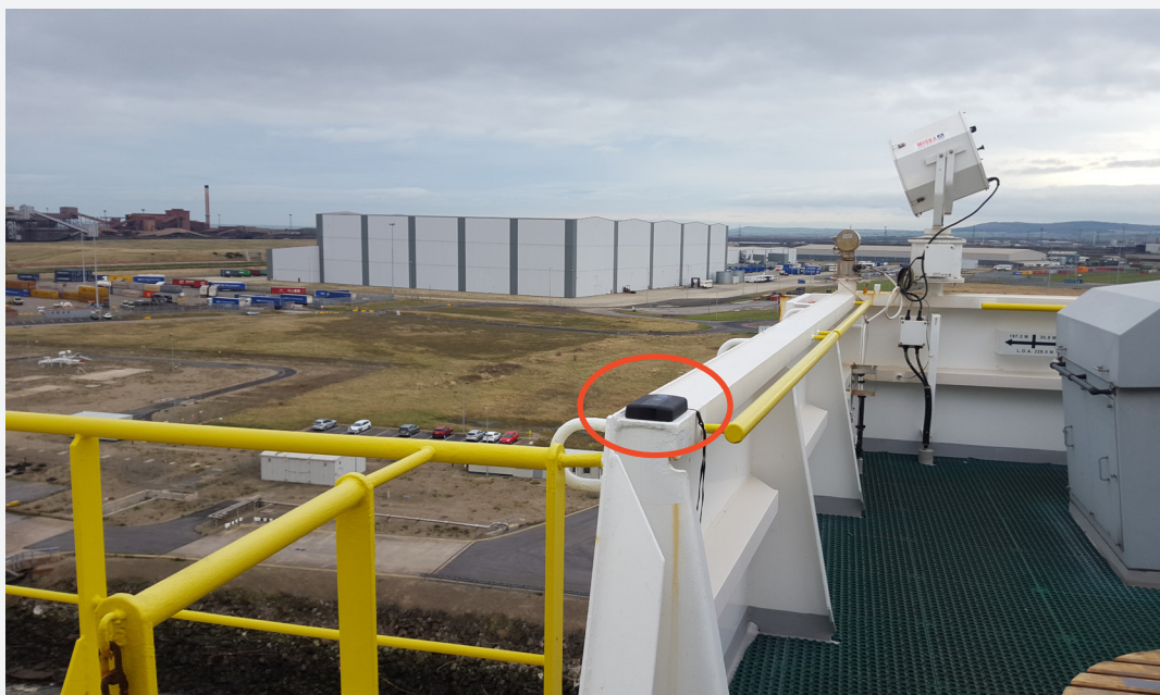
This is a very good location for the CAT XT GPS, as the area around the unit is clear and free of obstacles
