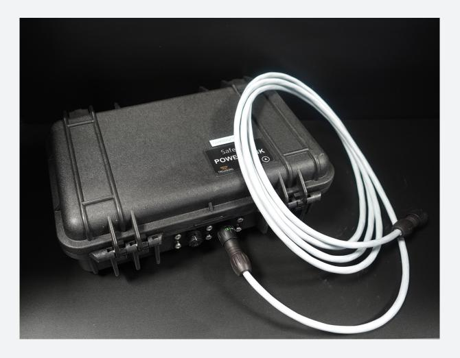
If needed during operation, to charge the CAT MAX, connect one end of the charging cable to the power bank and the other to the CAT MAX unit. Once the connection is made, the CAT MAX will begin charging, indicated by a blinking red light. This visual cue ensures the charging process is active and the unit receives power.
