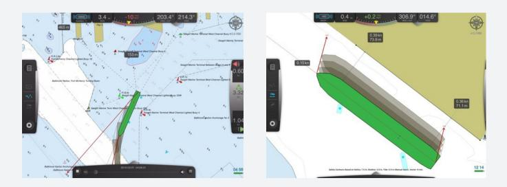
The SafePilot is a user-friendly software available as an app for iPad and Apple Watch. It handles key tasks such as navigation data, planning functions, route and arrival times, recording, chart handling, predictions, and history. Additionally, it offers specialized functions for docking and alignment, lock operations and weather data among other things.
