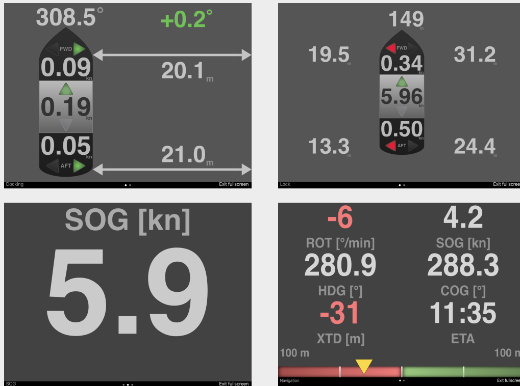
Figure 10.1: Some fullscreens: top left: docking, top right: in a lock, bottom left: simple navigation and bottom right: detailed navigation.
